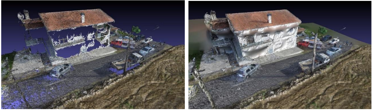
Figure 1 – Generated Point Cloud (left); Reconstructed Mesh (Right)
