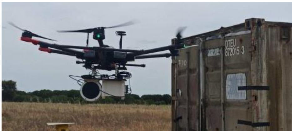
Figure 1 – Developed mobile radiation detection system coupled to a DJI Matrice 600 Pro multirotor for the inspection of a shipping container cargo. EJ-200 plastic detector (left side) and EJ-426HD detector with a HDPE moderator (right side).
