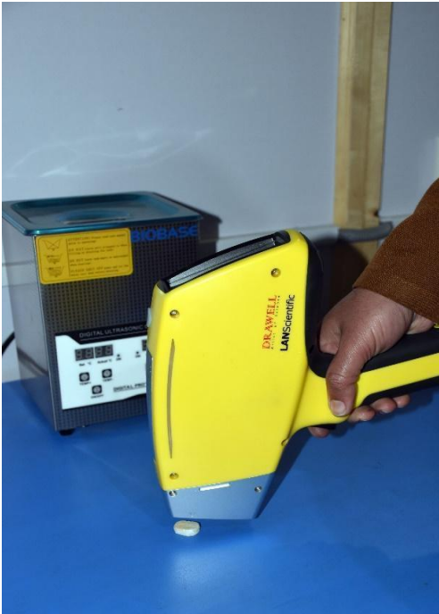
Figure 6- Portable XRF used in analyzing schist stones.
