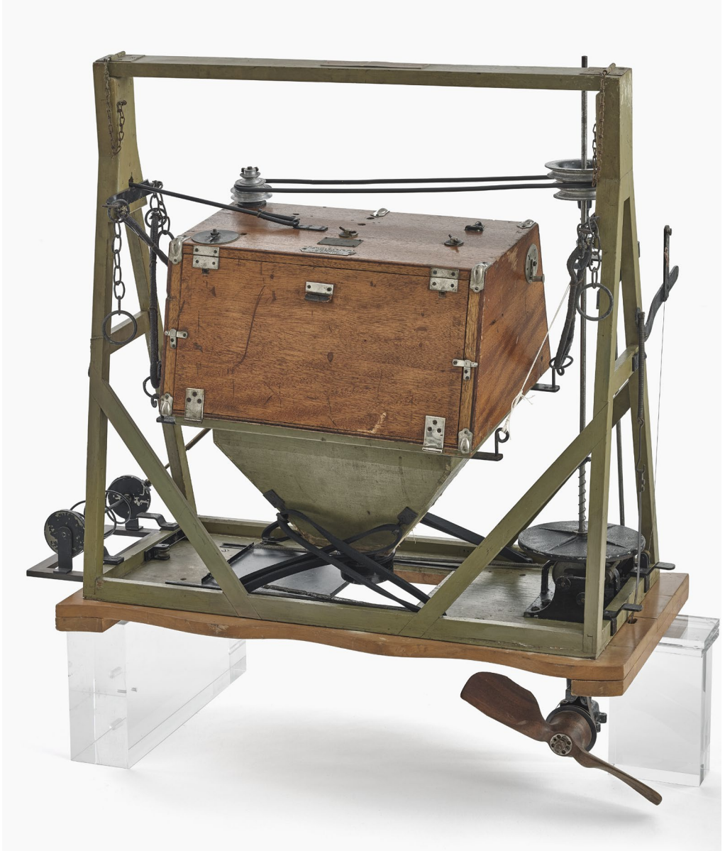
Fig. 1 Oskar Messter, film mapping camera Reihenbildner ("Rb I"), 1915, wood and metal, 890 × 860 × 400 mm. Munich, Deutsches Museum, Collection Photo- graphy-Cinematography, Inv. No. 56011 (56011_20220524_001_FotoraumSB_ND_ KRainer)
