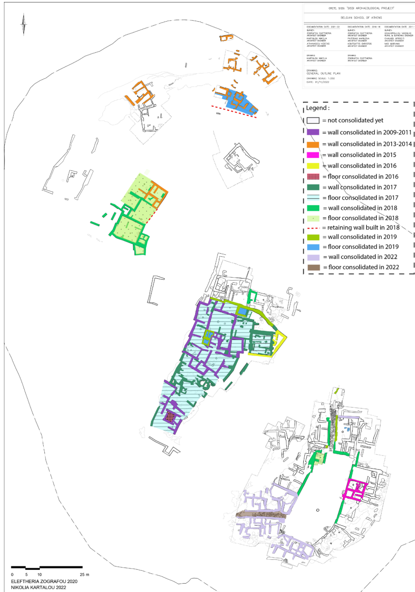
FIG. 24.3 SCHEMATIC PLAN OF THE KEPHALI HILL MAPPING THE DIFFERENT STABILISATION INTERVENTIONS PER YEAR (IMAGE T. CLAEYS, AFTER SITE PLAN BY E. ZOGRAFOU & K. NIKOLIA/© EBSA)
