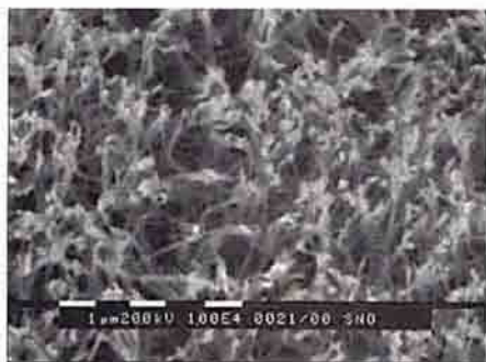
Figure 14. SEM image of a tin oxide electrode having a nanofibril morphology. The structure consists of nanodisperse 110-nm \text{SnO}_2 fibers protruding from a current-collector surface like the bristles of a brush. Reprinted with permission from [136], Li et al., J. Power Sources 97, 240 (2001). © 2001, Elsevier.
