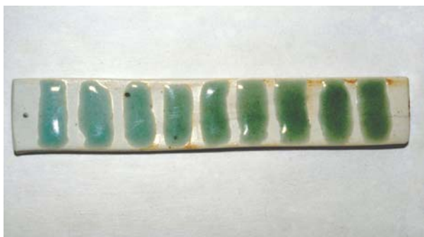
Figure 5. Effect of adding titanium dioxide to a lime-alkali celadon glaze containing 1.5% iron oxide (far left), up to 0.8% TiO 2 (far right), in 0.1 % increments. Reduction firing to 1250°C.
