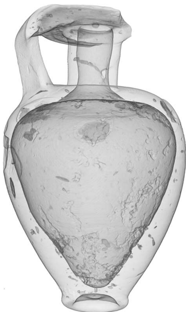
Figure 1. Protocorinthian Aryballos UMJ ARCH inv. 4214 (CT01184: 79 kV, 197 \mu A, voxel size 159 \mu m, Al 0.5mm), visualisation using the volume renderer developed at the VRVis Research Center, supported by ÖGI.
