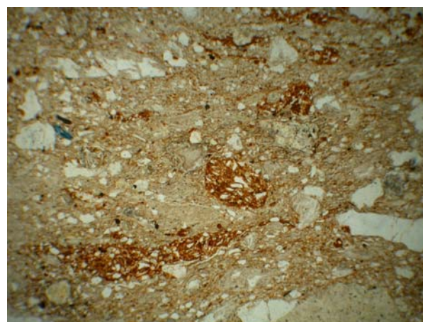
Figure 3. The presence of plastic, fabric-following argillaceous inclusions bands in tile specimen WLLQ-0061 (field of view = 2.5 mm).
