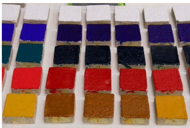
Figure 1: Some of the mock-ups subjected to the capillary rise cycles: samples are placed with the support in contact with filter paper soaked with distilled water.
