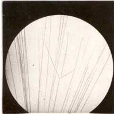
One of Blackett's photographs of particle tracks using the cloud chamber method. The forks show the collision of the particles with the nucleus of an atom. http://royalsociety.org/New-Theories-of-the-Atom
