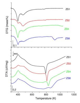
Fig. 1. DTA and DTG curves for the supports.
