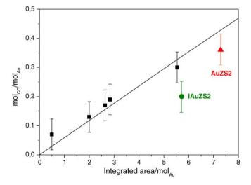
**Fig. 5.** CO chemisorbed amounts vs. integrated intensities of the FTIR CO bands normalised to the gold content for the AZS2 (triangle) and IAZS2 (circle) samples in comparison with a series of Au/ZrO<sub>2</sub> catalysts (square).
