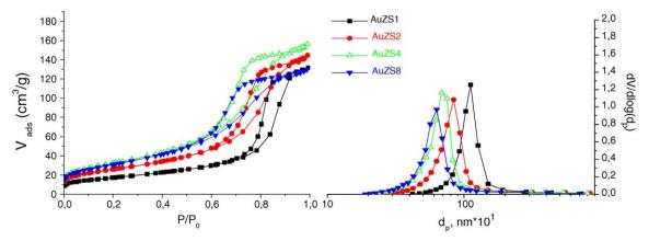
Fig. 2. N<sub>2</sub> physisorption isotherms and BJH pore size distributions of catalysts.
