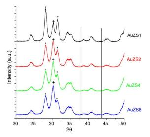
Fig. 3. XRD patterns of catalysts (★) monocline zirconia and tetragonal zirconia (+).
