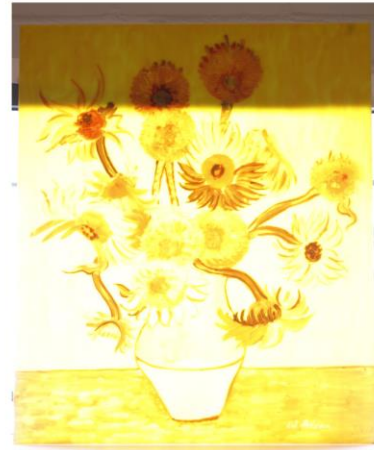
(c) Volume-based colour reproduction using Stratasys J750
