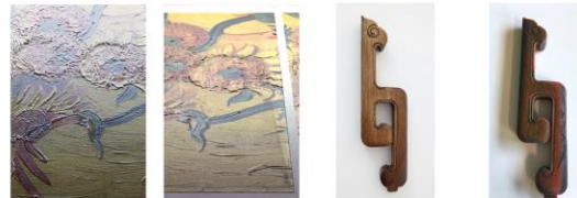
4(a) Surface based colour reproduction with spatially-varying surface gloss, using Océ Technologies High Resolution 3D printing 6(a) Original part: Part of traditional Chinese table (b) Volume-based colour reproduction using Stratasys Connex3
