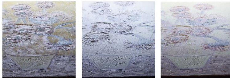
3. Mirror angle illumination (a) Original painting: Sunflowers in the style of Van Gogh (b) Surface based colour reproduction using Océ Technologies High Resolution 3D printing (c) Volume-based colour reproduction using Stratasys J750
