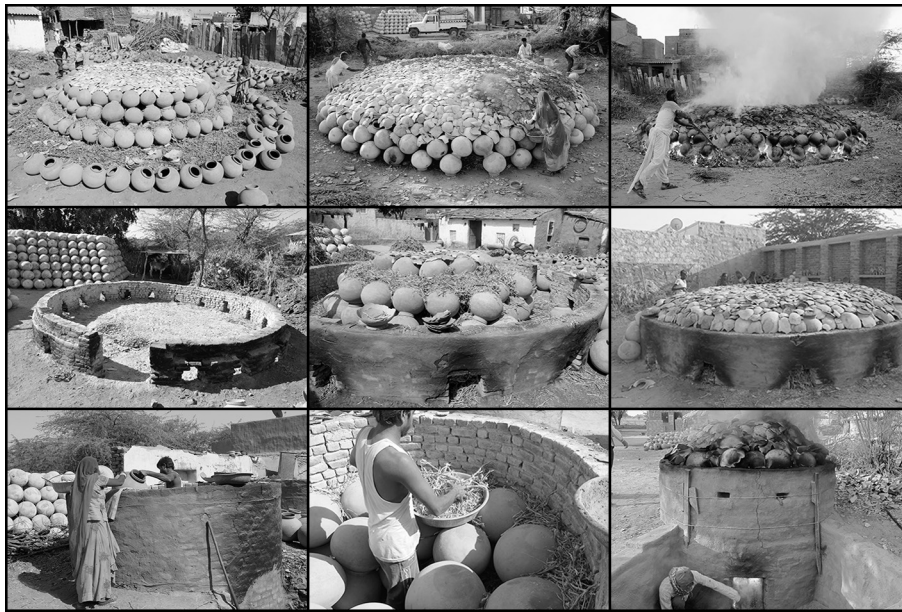
FIG. 2.1 THE DIFFERENT FIRING STRUCTURES USED BY THE POTTERS IN PACHPADRA: (TOP) OPEN MULTIPLE-HEARTH CIRCULAR FIRINGS, (MIDDLE) ENCLOSED MULTIPLE HEARTS CIRCULAR FIRING, (BOTTOM) VERTICAL UPDRAFT KILN (©VALENTINE ROUX)
