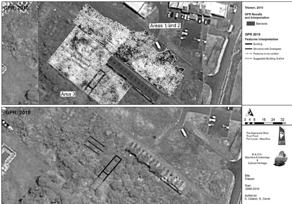
Fig. 6: Ground Penetration Radar (GPR) results and interpretation, 2010
