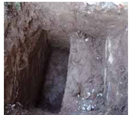
9. Excavation pit for collecting undisturbed soil sample
