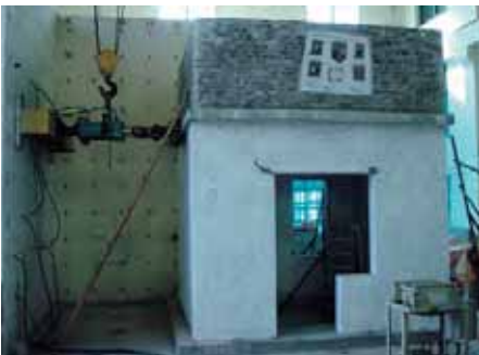
16. Quasi static test of full scale room retrofitted with ferrocement
