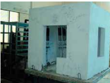
15. Shake table test of one room model retrofitted with ferrocement
