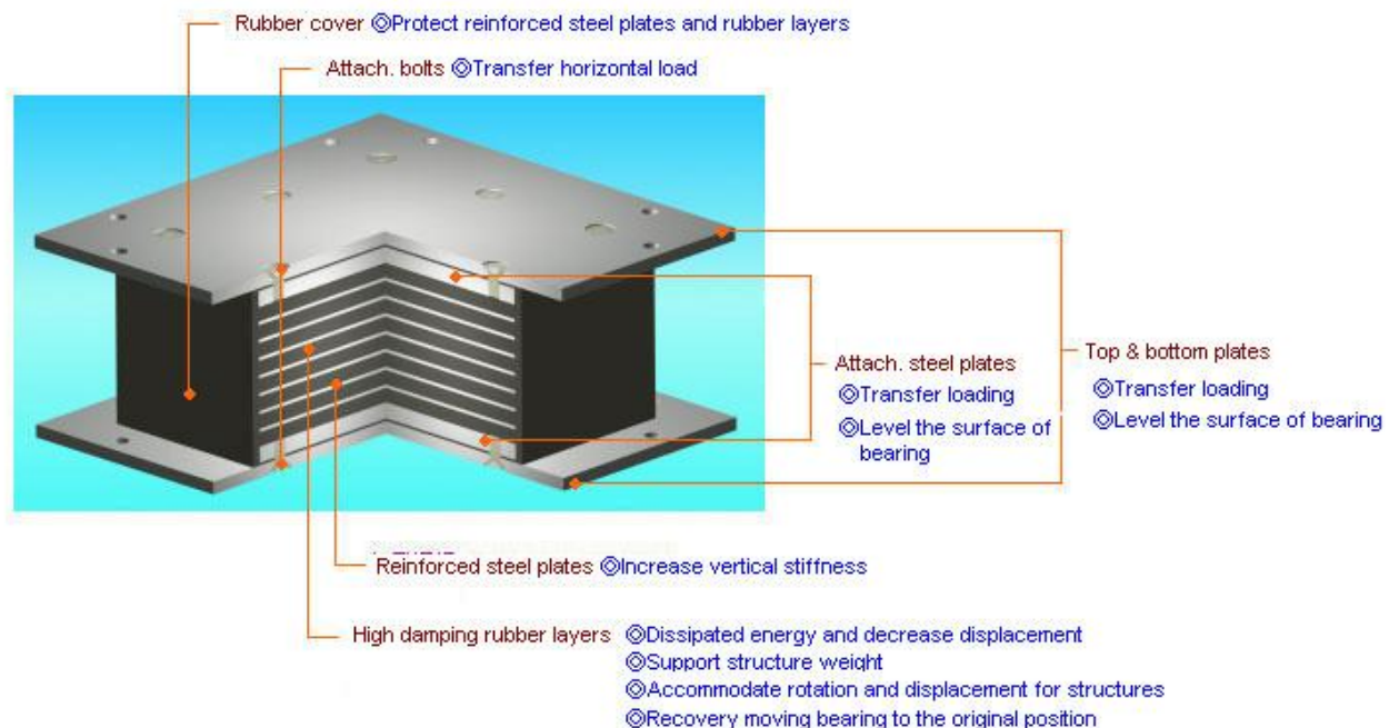
Figure 26: Structure of High Damping Rubber Bearing (HDRB) (photo: Official Website Lien Foo Rubber Products Company)
