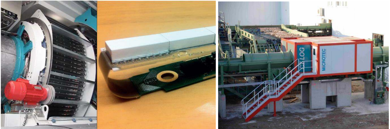
Figure 1 - Internal view of the scanner, with the sensors mounted on the black bars in the gantry (left); one of the sensor modules developed by Microtec (center); one of the sawmill installations of the scanner (right).
