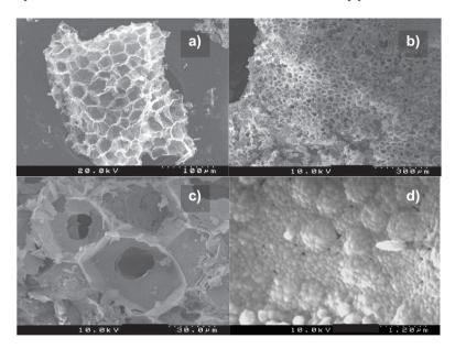
Fig. 2. SEM images of a) cork pyrolised under Ar at 900 °C, b)-d) pure CeO<sub>2</sub> ecoceramics, after heating at 1000 °C in air, with the cellular structure of the cork template. Image d) shows the nanoscale nature of the constituent grains of this ecoceramic.
