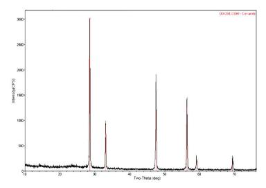
Fig. 3. XRD pattern of the CeO<sub>2</sub> ecoceramics heated to 1000 °C / 2 hr. The peaks shown are, from left to right, (111), (200), (220), (311) and (400), and the standard used is JCPDF 00-034-0394.
