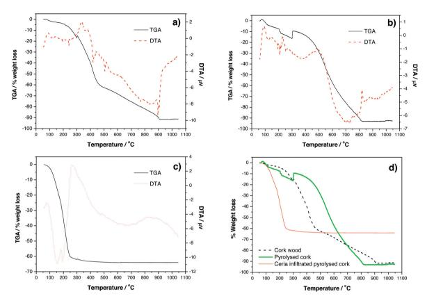
Fig. 1. DTA-TGA plots for a) cork wood powder, b) previously pyrolised cork powder, c) ceria precursor infiltrated pyrolised cork powder. The % weight loss of all three is directly compared in d).
