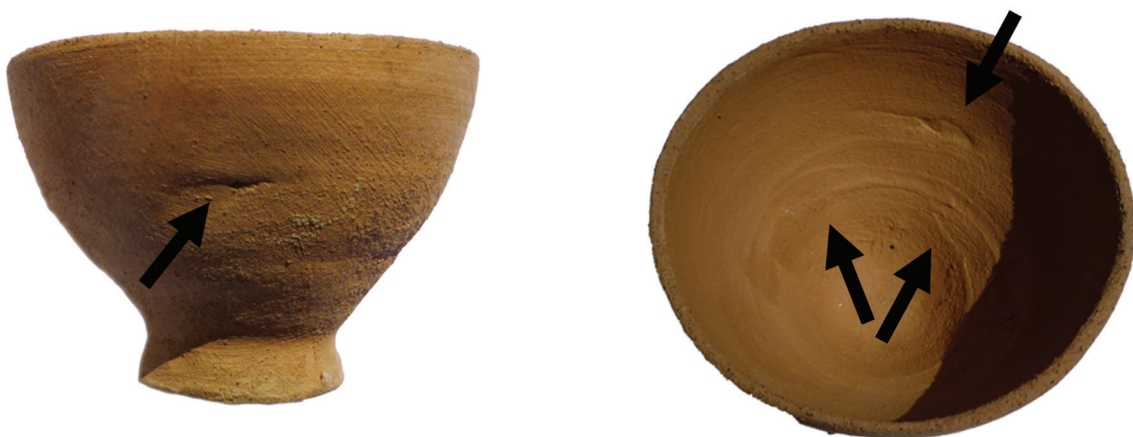
Figure 7. Handleless conical cup reproduced by V. Politakis using wheel-coiling with arrows indicating a deep horizontal fissure on the outer face (left), and curvilinear fissures and compression folds on the inner face (right). Photograph by author.
