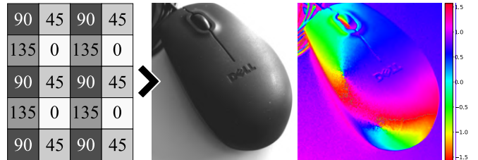
Fig. 1. Our method demosaics a PFA camera image to produce a high-resolution intensity image (center) and angle of polarisation (right).
