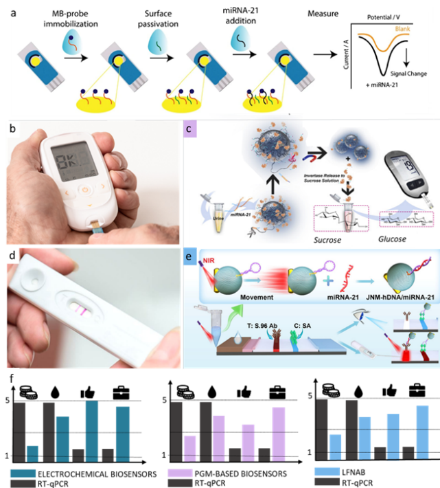
Figure 3. (a) Electrochemical biosensor for miRNA-21 based on an amperometric readout adapted from [33]. (b) Example of commercial PGM. (c) PoC biosensor for the detection of miRNA-21 in urine obtained combining functionalized magnetic beads and PGM adapted from [34] (Copyright permission n. 55946915111809). (d) Example of LFA for COVID-19 screening. (e) LFST with a dual readout including near-infrared-powered nanomotors for the detection of miRNA-21, adapted with permission from [35] Copyright 2023 American Chemical Society. (f) Comparison of the discussed PoC for miRNAs in terms of costs (symbol: coins), sample values (amount of sample required; symbol: drop), user-friendliness (symbol: thumb up) and portability in a scale from 1 to 5 (symbol: hand bag). For portability and user-friendliness, 1 is poor and 5 optimal. For costs and sample amount, 1 correspond to a low value and 5 to a high one.
